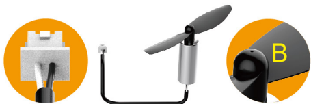
★ B: CCW motor with black&white wire
